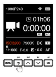
Shutter Speed / Angle: Press UP to set shutter speed / angle (refer to 2.5
