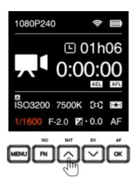
• **EV**: Press **DOWN** to set EV, then press **Up** / **Down** to adjust the value, and **OK** to confirm.
