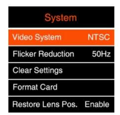
Video System: NTSC / PAL / CINEMA. Different frame rates in Video Format for recording and frame rates in VFR\* for capturing are supported by these three Video System as below:
