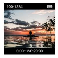
When the footage is being played, press **OK** button to pause / resume, and press **MENU** button to stop it.
