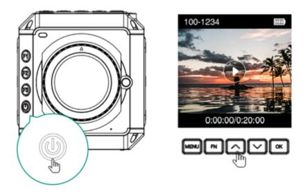
Press **OK** button to play the selected footage. When the footage is being played, press the **Up** / **Down** button to speed up / slow down (2x faster / slower).
