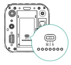
**Single (I)**: The camera is working as an individual device.
