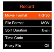
Movie Format: It's resolution & frame rate for video recording. Please note that the camera support three video systems including NTSC, PAL and CINEMA (2.10 System – Video System). Movie formats for each video system are as below:
