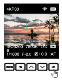
Aperture: Press F3 to set the aperture, then press Up / Down to adjust the value, and OK to confirm. Please note that F3 can be assigned to other quick settings besides Aperture (2.10 System – Fn)
